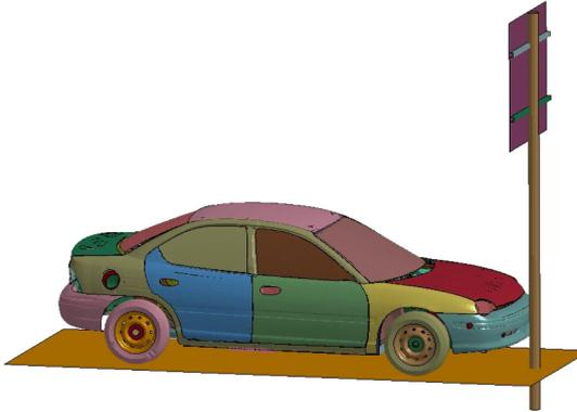
**Fig. 1.** Crash Simulation Model.
