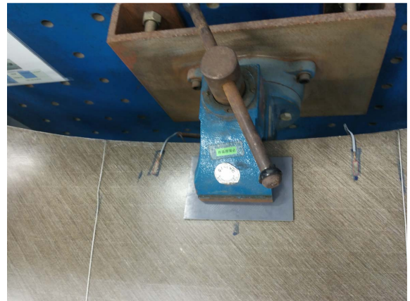
Fig. 11. Bonnet mounting and attachment of strain gauge
