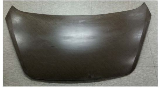
Fig. 10. Manufactured prototype of automobile bonnet
