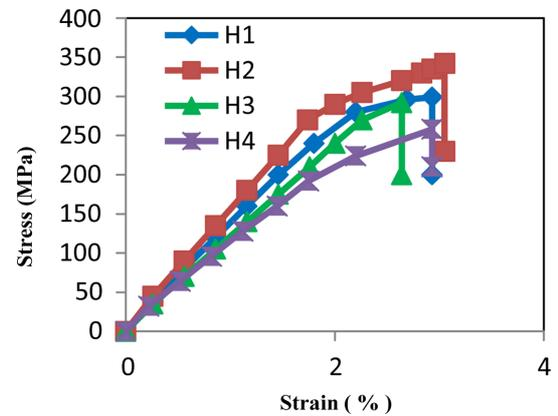
Fig. 4. Stress-strain curves for basalt carbon inter-ply hybrid composites with different angle ply orientation
