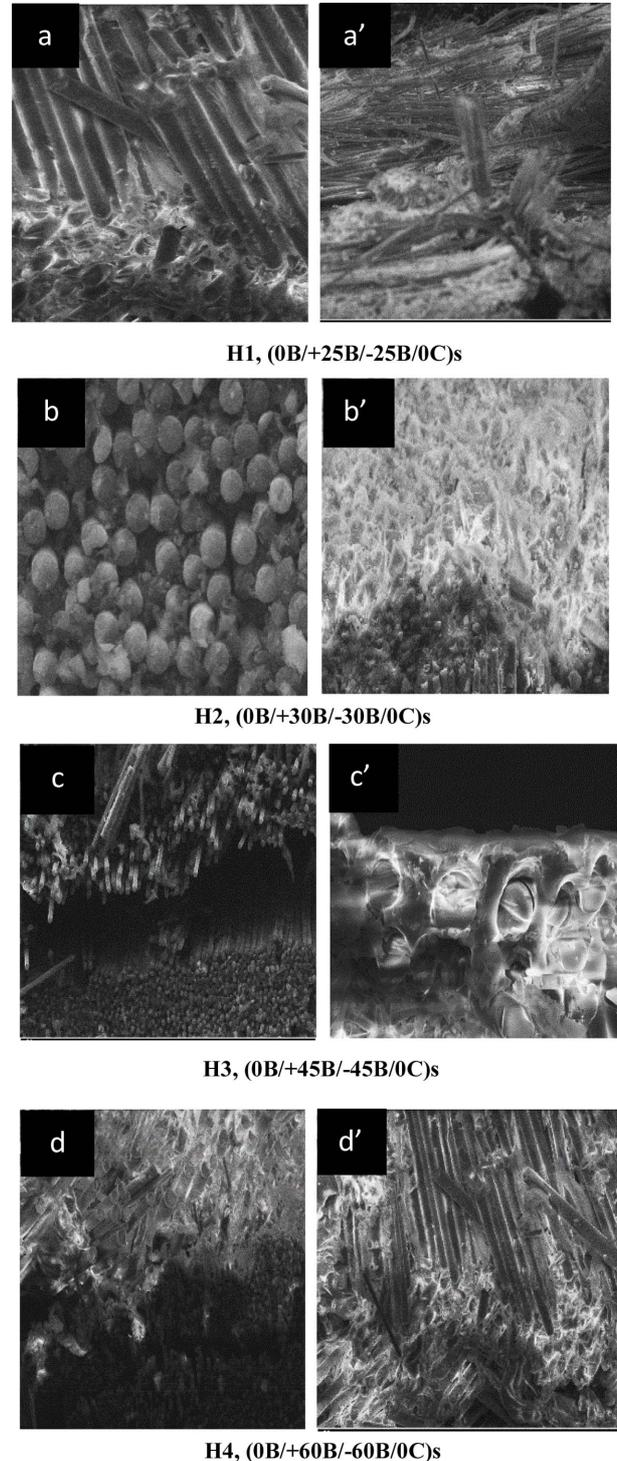
**Fig. 7.** SEM images of the cross-section of the fractured surfaces of basalt carbon hybrid composites with different angle ply orientation
