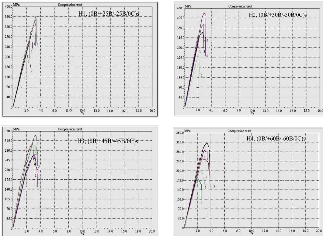
Fig. 3. Experimental scatter curves for basalt carbon inter-ply hybrid composites with different angle ply orientation
