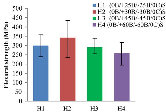
**Fig. 5.** Average flexural strength for basalt carbon inter-ply hybrid composites with different angle ply orientation
