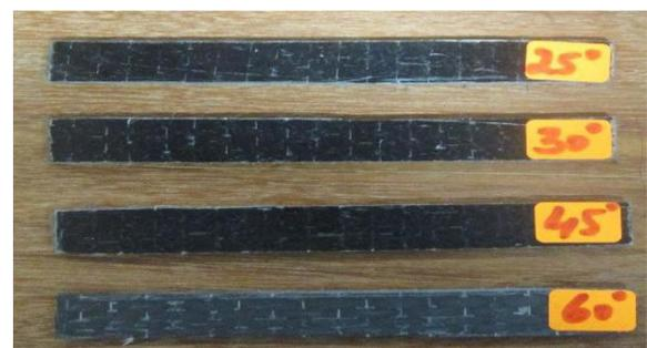
**Fig. 1.** Basalt carbon hybrid composite specimen with different orientations
