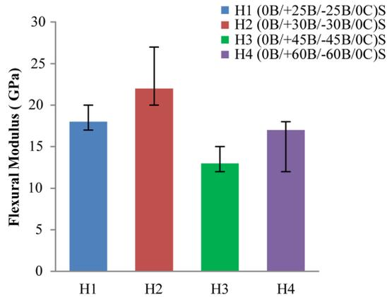
**Fig. 6.** Average flexural modulus for basalt carbon inter-ply hybrid composites with different angle ply orientation
