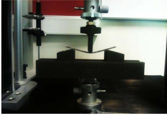
Fig. 2. Test specimen in three point bending mode
