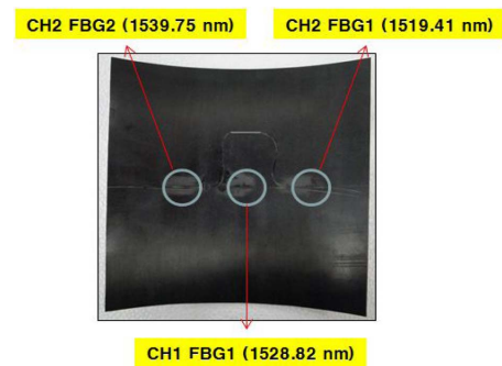
Fig. 6. Three FBG sensors attached to the composite shell
