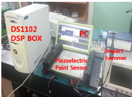
Fig. 4. Experimental setup for impact test
