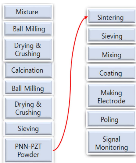
Fig. 1. Manufacturing process of the piezoelectric paint
