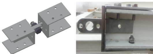
Fig. 9. Previous connection system between unit structures
