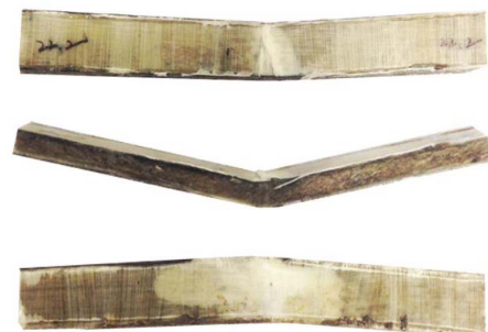
Fig. 7. Composite specimen after three-point bending test
