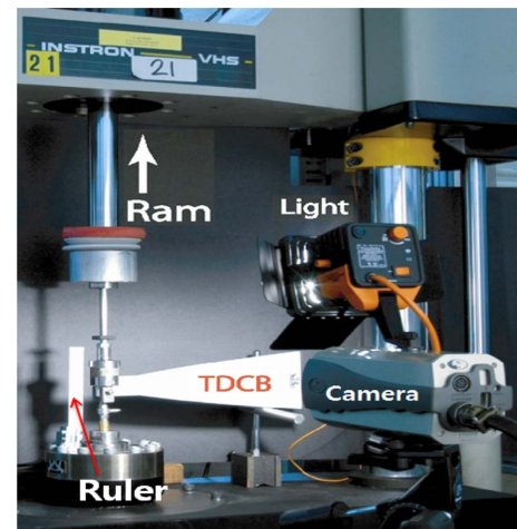
Fig. 3. Setup of aluminum alloy at impact tester
