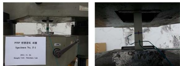
Fig. 4. Tensile test (Pultruded FRP)
