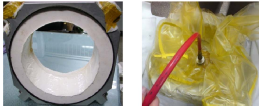
Assembly of inner mould and Degassing
