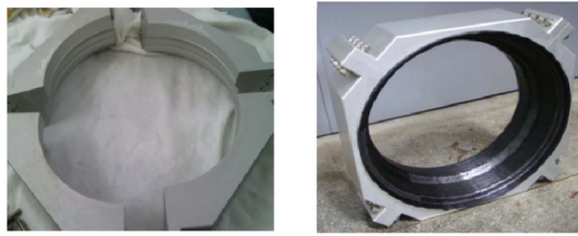
Assembly of Al-mould and Composite stacking
