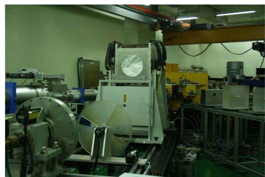
Fig. 9. CNT/E and Gr/E coupons for TID test
