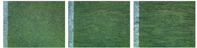
Fig. 6. CNT inclusions alignment in a uniform electric field (5Hz, 4.5 kV/mm, \times 1200 magnification)
