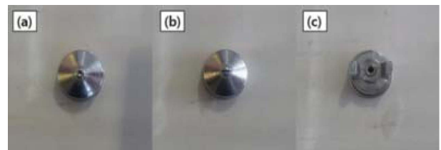
Fig. 2. Three different types of the spray nozzle hole shape.
