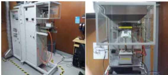
Fig. 9. Cone calorimeter test.
