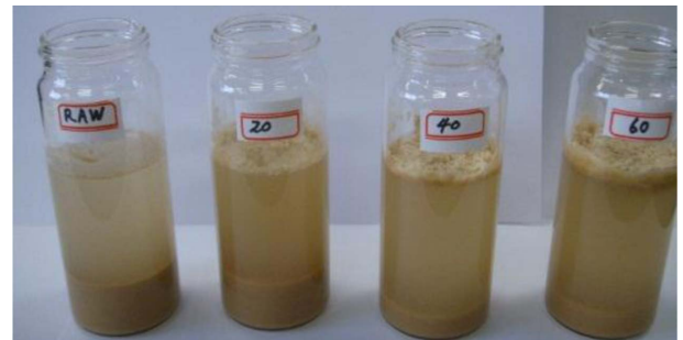
Fig. 4. Wood powder precipitation test.
