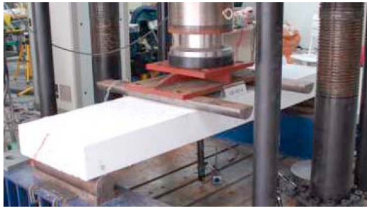
Fig. 2. 4-points bending test.
