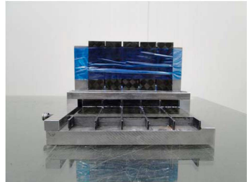
Fig. 3. Bonding assembly tool for L-type specimen.
