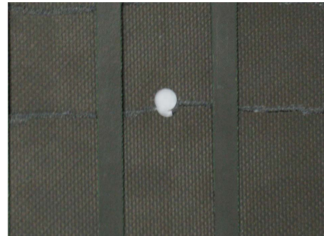
Fig. 16. Fatigue damage crack growth pattern for stiffened panel.
