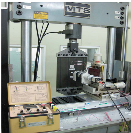
Fig. 15. Test set-up for stiffened panel.
