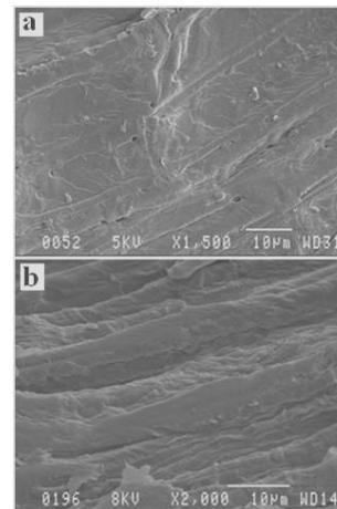
**Fig. 2** SEM photographs of Untreated (a) and alkali treated (4 h) (b) *Borassus* fruit fine fibers.**Table 2** Chemical composition of untreated and alkali treated *Borassus* fruit fine fibers
