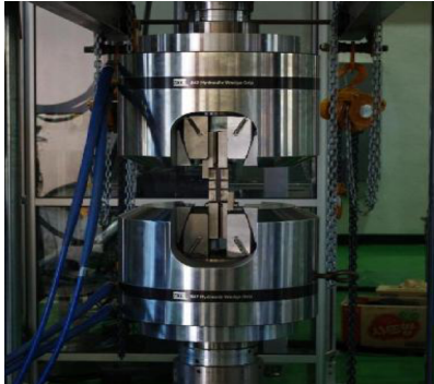
Fig. 4 Compression test after damage.
