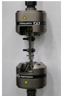
Fig. 4 Double lap key joint.
