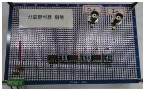
Fig. 1 Photograph of the OP amp.
