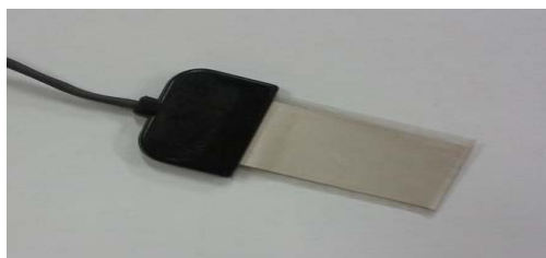
Fig. 2 Photograph of the PVDF sensor.
