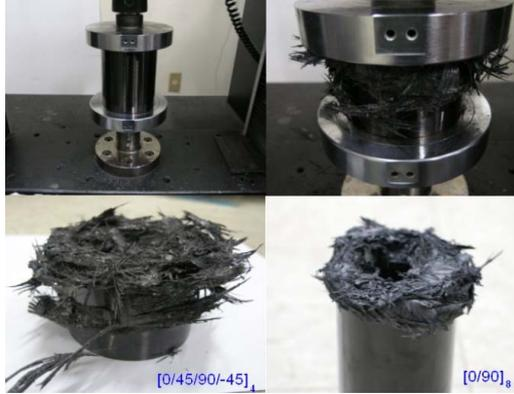
Fig. 4 Quasi static tests set up and results.
