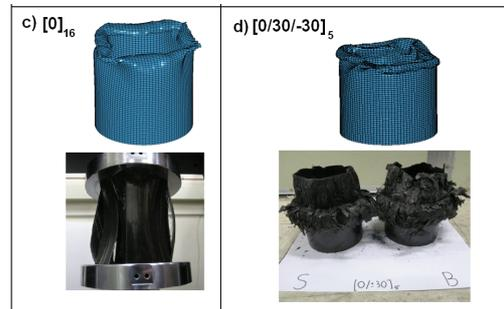
Fig. 14 Final stage of the specimens (S: notch, B: bevel).
