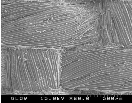
Fig. 12 SEM photograph of glow plasma treated fabric after adhesion test.
