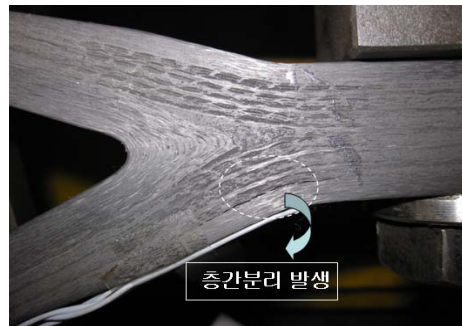
Fig. 15 Onset of Delamination Failure.
