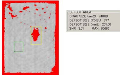
a) A defect area of B-787 sample
