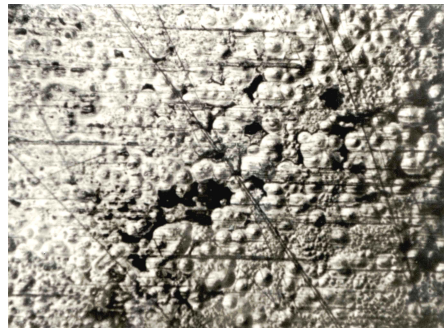
(c) Surface of air-cooled moldings
