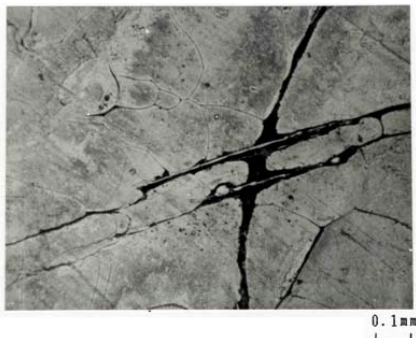
Fig. 7 Fiber exposure and micro weldline.
