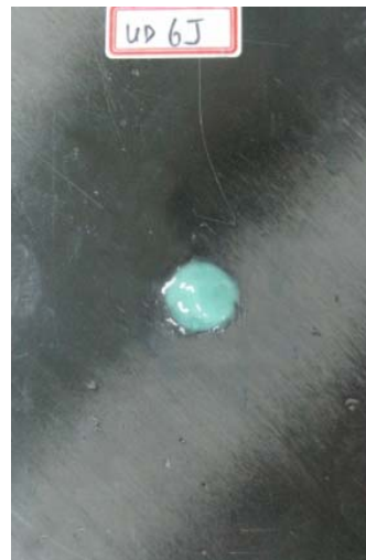
Fig. 9 Application of adhesive on removed area.
