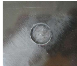
Fig. 8 Removal of impact damaged zone.
