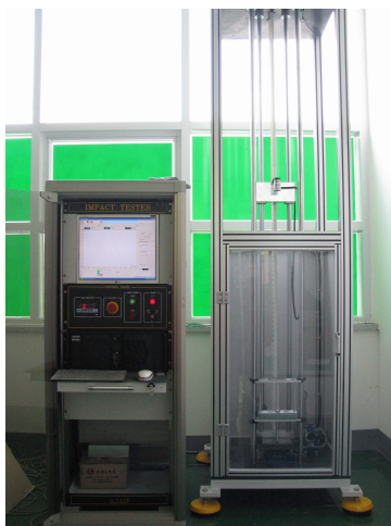
Fig. 3 Impact test equipment.
