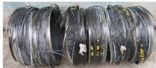
Fig. 14 Failure mode of \phi 157.0(mm) hoop ring.
