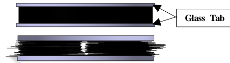
Fig. 7 Failure mode of reinforced hoop ring.
