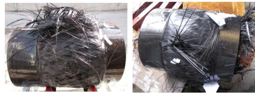
Fig. 9 Typical cylinder Failure mode from hydro-burst test with Ø 500.0(mm) vessel.
