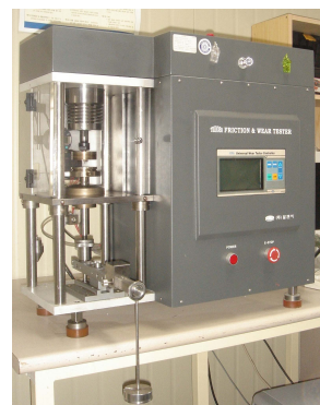
Fig. 3 Pin-on-disk friction and wear tester.
