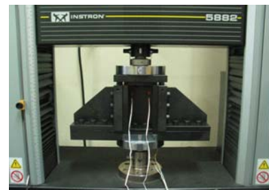
Fig. 4 Test jig for CAI
