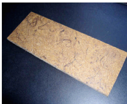
Fig. 4 The coir/rubber composite board [23].
