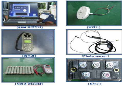
Fig. 27 Equipment for the blade performance test
