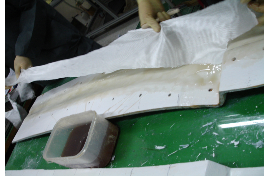
Fig. 20 Lay-up process on the mold.
