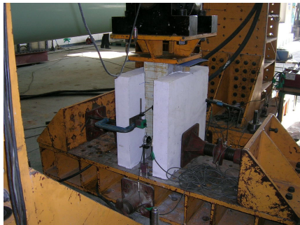
Fig. 11 Push-out Test.
