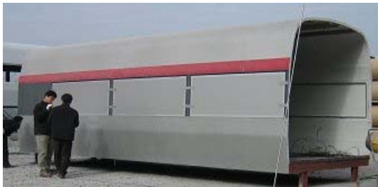
Fig. 4 Test carbody for the fire safety evaluation.
