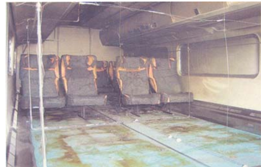
Fig. 8 Inside of the tested composite carbody with interiors.
