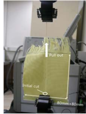
Fig. 12 Yarn pull-out test setup
