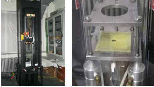
Fig. 7 Drop testing machine(Instron Dynatup 8250) and air pressurized jig
