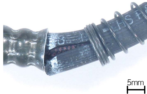
Fig. 7 Fractured part of the rubber hose assembly.
