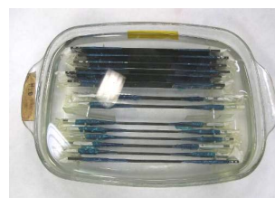
(a) USN175B 0° and Fabric Tensile Specimen
