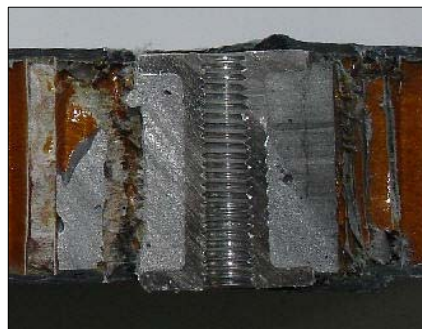
(b) Shear Failure
