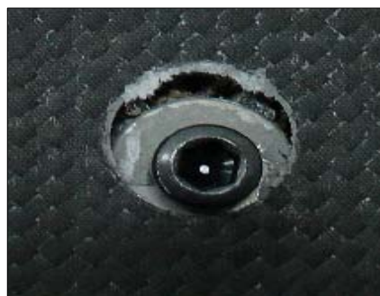
(a) Pull-out Failure
