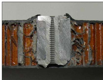
(a) Pull-out Failure
