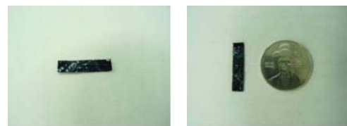
Fig. 1 Photos of PANi film samples.
