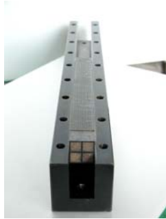
Fig. 9 Fabrication procedure of the sandwich column with a mould.
