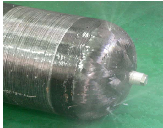
Fig. 14 Leak around knuckle part after failure by pressure cycling test of composite cylinders.
