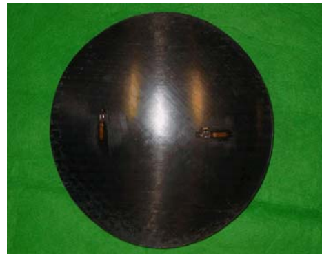
Fig. 13 The final product with strain gauges attached on the surfaces.
