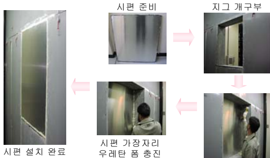
Fig. 2 Installing Procedure of Specimen.
