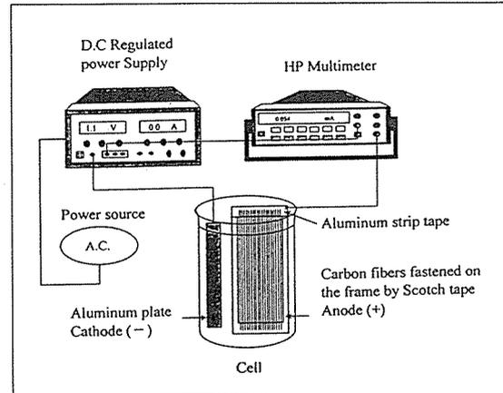
Fig. 1. Schematic plot of electrodeposition (ED) system
