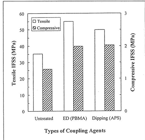
Fig. 6. IFSS for two coupling agents compared to the untreated case
