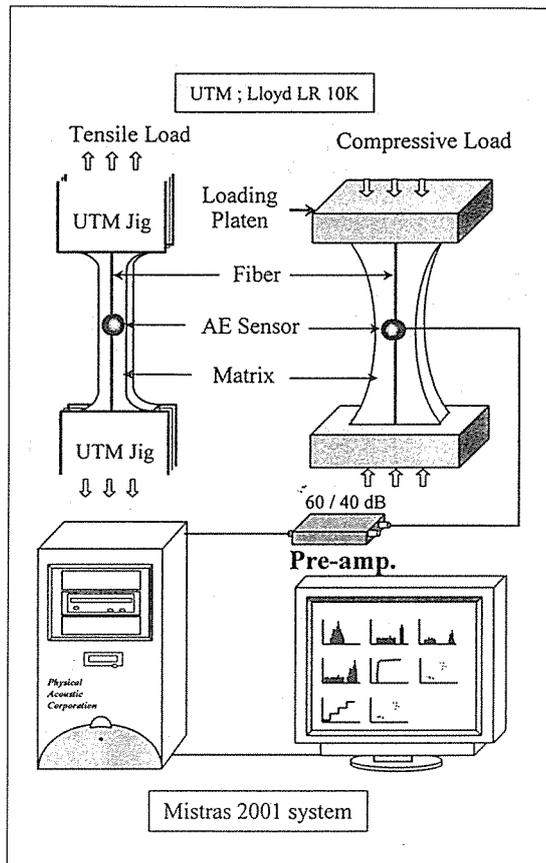
Fig. 4. Schematic diagram of instrumentation for AE
