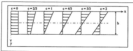
Fig. 2 Numerical factor c for bending stresses
