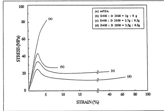
Fig. 5. Plot of stress-strain curve for the dogbone-shaped epoxy specimens using four different curing agents: (a) *m*PDA; (b) D400 : D 2000 = 3g : 0 g; (c) D400 : D 2000 = 2.7g : 0.3g; (d) D400 : D 2000 = 2.5g : 0.5g.
