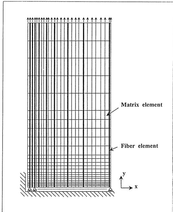
Fig. 12. Finite element mesh. (This is an example in the case that a support is removed at the second-arrayed fiber from the left.)
