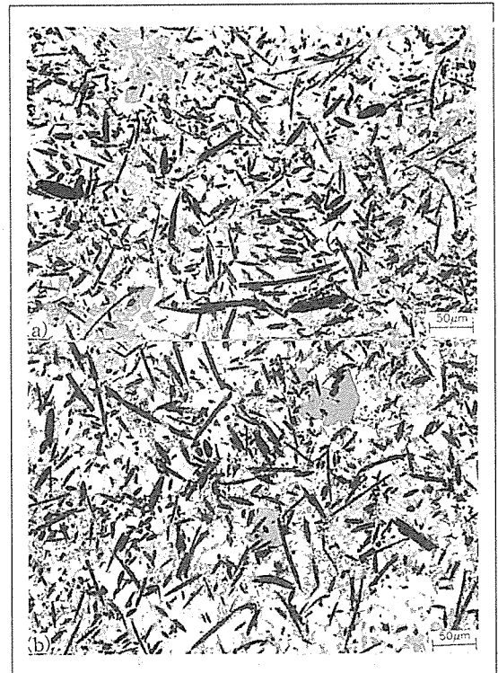
Fig. 7. (a)(b) Optical micrographs of MMCs along the longitudinal direction in the cross section perpendicular to pressurizing direction ( T_p=300^\circ\text{C} , T_m=400^\circ\text{C} , V_f=10\% , T_i=800^\circ\text{C} , P=75\text{MPa} )
