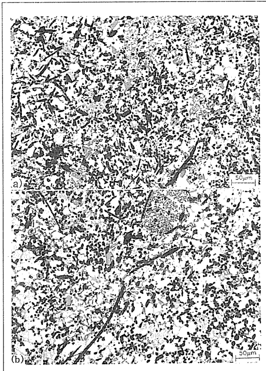
Fig. 6. (a)(b) Optical micrographs of MMCs along a direction parallel to the pressurization ( T_p=300^\circ\text{C} , T_m=400^\circ\text{C} , V_f=10\% , T_i=800^\circ\text{C} , P=75\text{MPa} )
