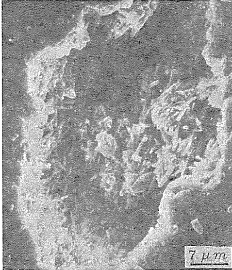
Fig. 12 Scanning electron micrograph of the residual pore in the Al-SiCw composite billet consolidated at the condition of 600°C/50 MPa, showing the agglomeration of SiC whiskers.
