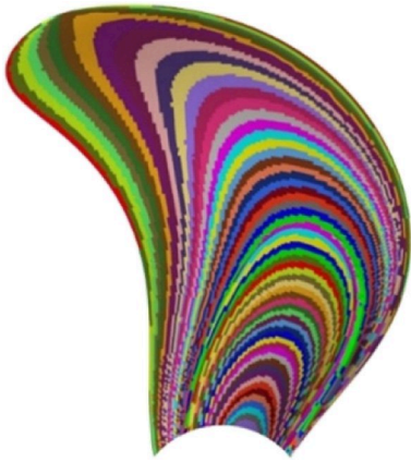
Fig. 8. Resulting FE model incorporating a continuously varying laminate configuration
