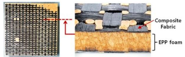
Fig. 6. [fabric/EPP/fabric] sandwich panel and its cross section view
