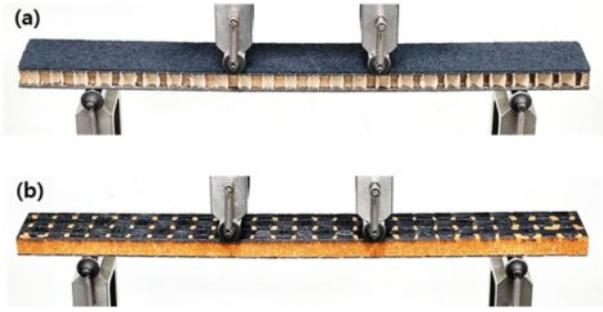
Fig. 11. 4-point bending test of sandwich panel specimens; (a) GMPUR panel, (b) [fabric/EPP/fabric] panel
