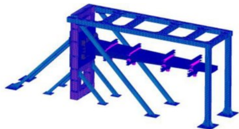
Fig. 11. FE models of torsion box and test fixture
