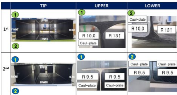
Fig. 7. Fabrication for 1.5 m torsion box module
