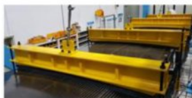
Fig. 20. Test fixture assembly for static structural test
